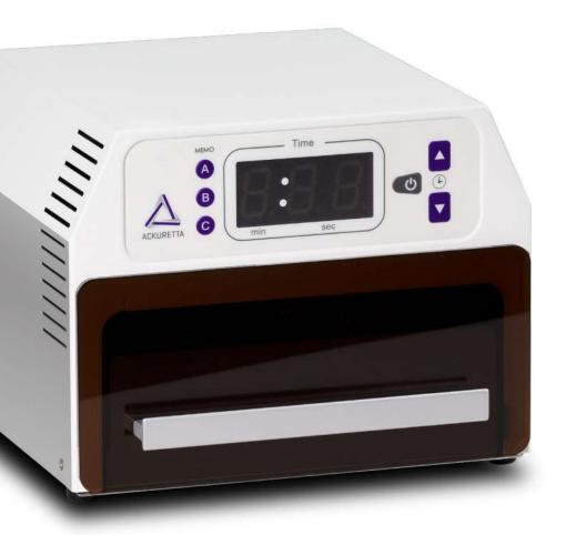
The Ackuretta UV Box is a compact curing box lined with long-life ultraviolet LED bulbs for enhanced curing performance. The reflective stainless steel chamber and bottom mirror surface provides even curing to all sides. The UV Oven is designed with two modes, continuous and flash (10 flashes/second), to ensure all resins that react to wavelengths 365, 385, and 405nm can cure completely and efficiently, with strengthened print hardness. It is also suitable for Class I materials.
